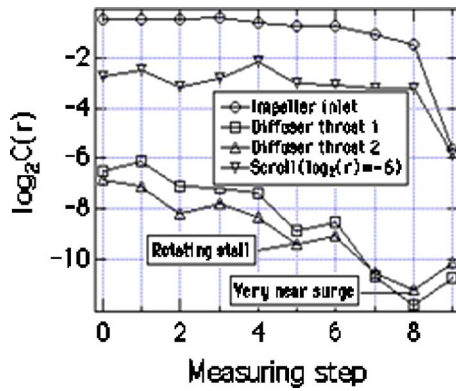
Fig. 9 The correlation integrals around surge at four positions (FP vanes, 50,00 rpm)
