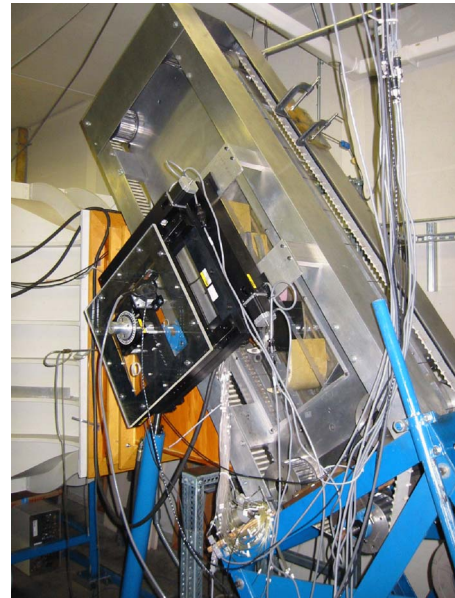
Fig. 3 Turbine cascade research facility with three-axis traversing system
